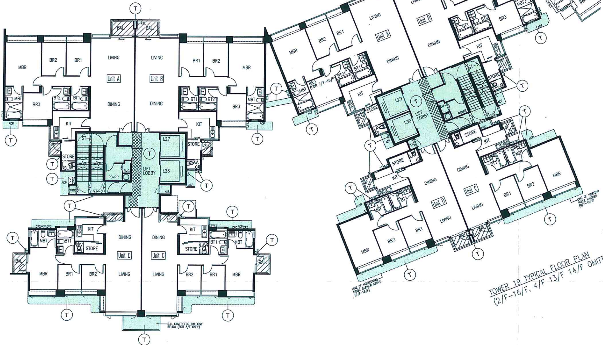
TOWER 18 TYPICAL FLOOR PLAN (2/F-16/F, 4/F 13/F 14/F OMITTED)
